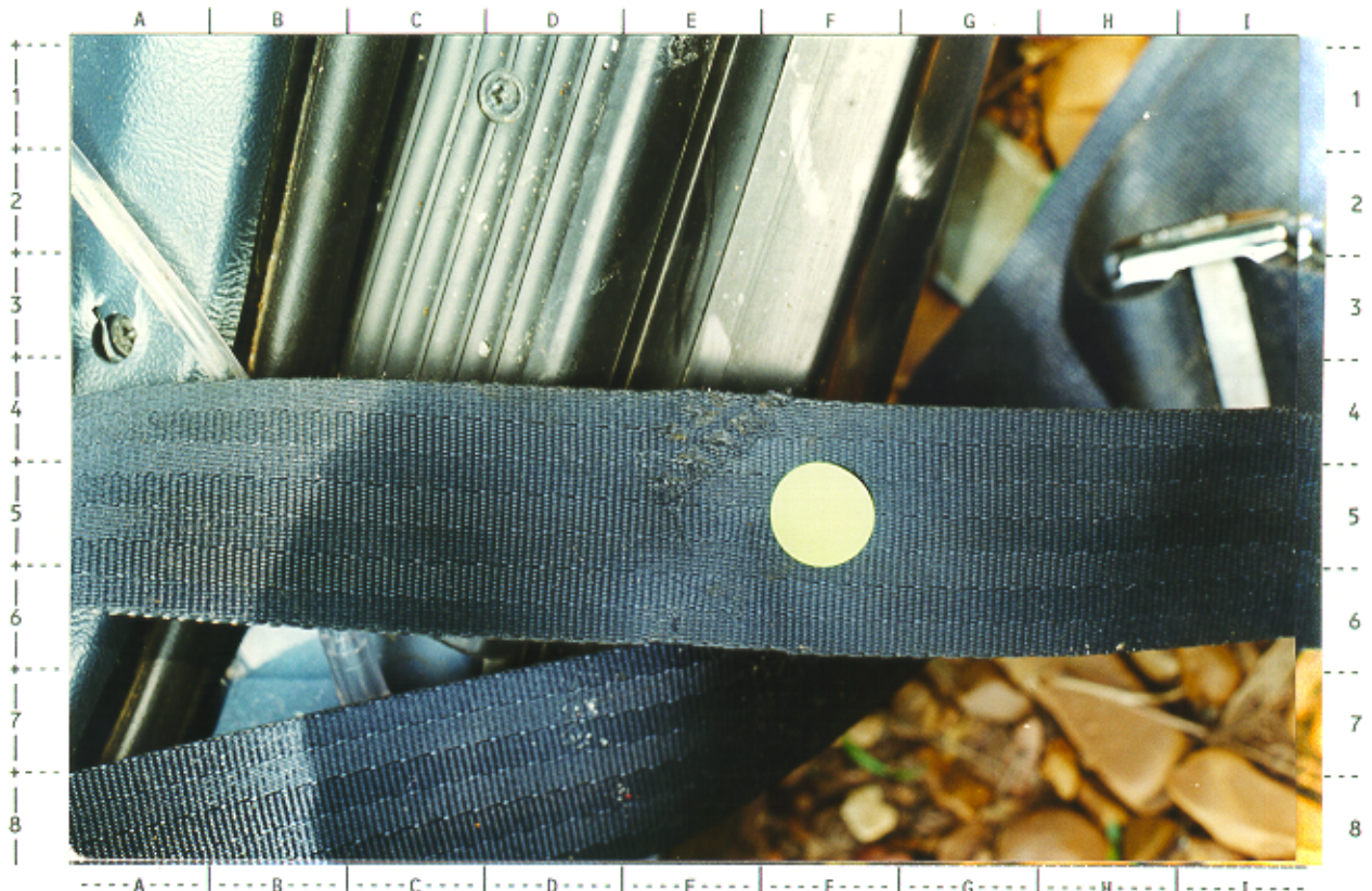
# 60 -- Stress marks present on torso portion of '91 Chevrolet Corsica's driver seat belt; see cells D4--E5
